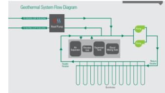
A 7-unit heat pump in the main mechanical room operates in either a heating mode or a cooling mode. The system is designed to provide heating using the natural thermal energy in the ground for the majority of the heating season. When temperatures fall in the range of -10 °C to -5 °C, the heating needs within the building will exceed the design of the system and natural gas boilers will be used to meet the heating demand.
