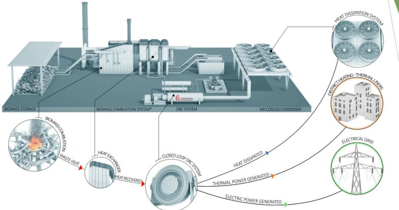
HEAT TRANSFER FLUID The heat from biomass combustion is transferred to the ORC working fluid by means of an intermediate circuit or directly via the combustion gases in direct exchange systems. The media used in the intermediate circuits are thermal oil, saturated steam or superheated water.
