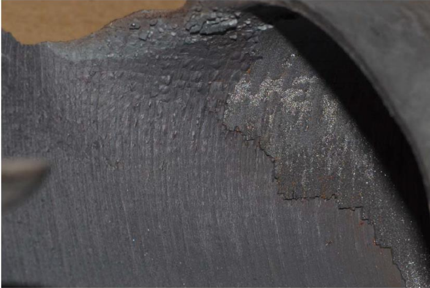
Fissures and Oxide Layer on ID of Tube
