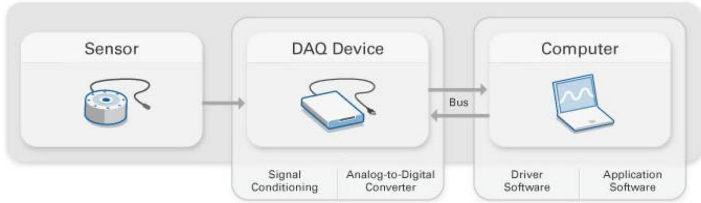
**Data acquisition (DAQ)** is the process of measuring an Thermal or physical phenomenon such as voltage, current, temperature, pressure, or sound with a computer. A DAQ system consists of sensors, DAQ measurement hardware, and a computer with programmable software.
